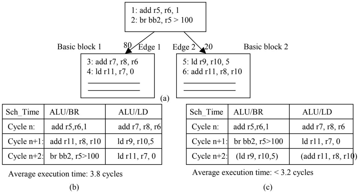
Figure 2. (a) An example for treeregion scheduling, (b) the scheduling result using list scheduling, (c) the scheduling result using TTS
