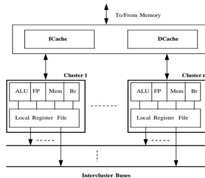
**Figure 1. A sample clustered microarchitecture. Current similar microarchitectures include the Alpha 21264 and the TI TMS 320C6x. The disjoint nature of the register files complicates instruction scheduling.**
