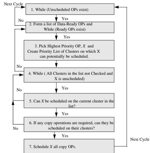
Figure 3. A framework for implementing unified assign and schedule(UAS).
