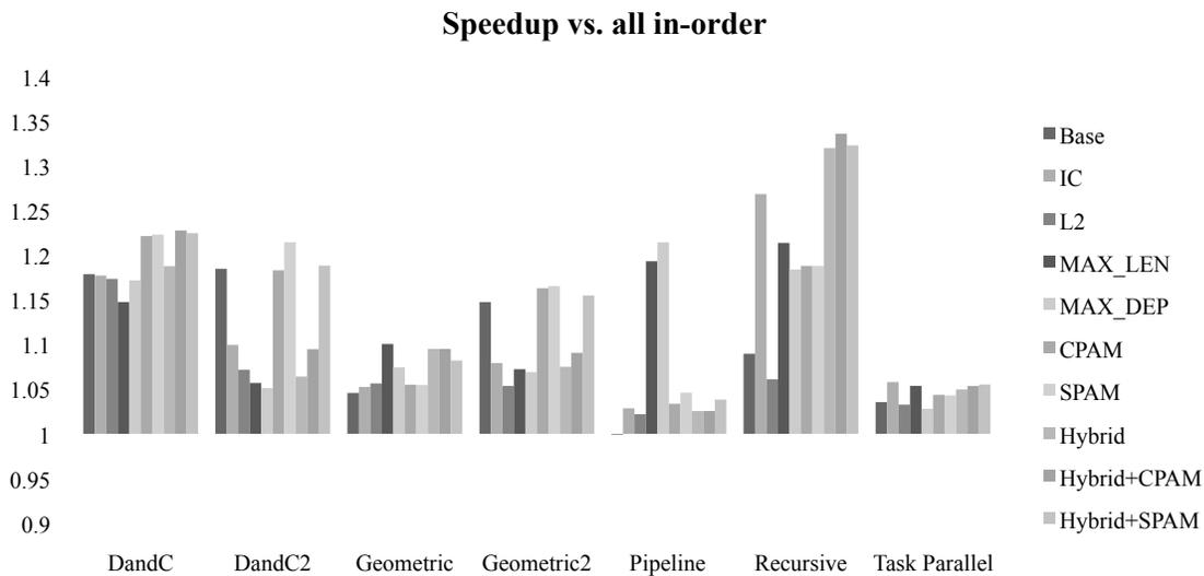
**Figure 7** - Speedup results for pattern-centric microbenchmarks
