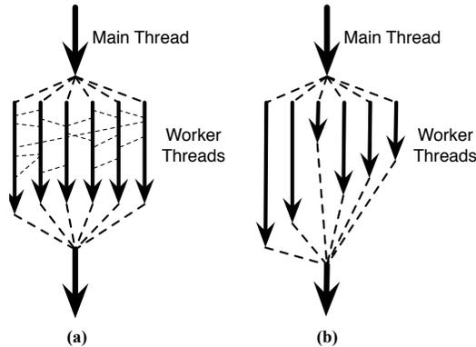
**Figure 3** - Thread Behavior of Data Centric Patterns (a) Geometric Decomposition (b) Recursive Data
