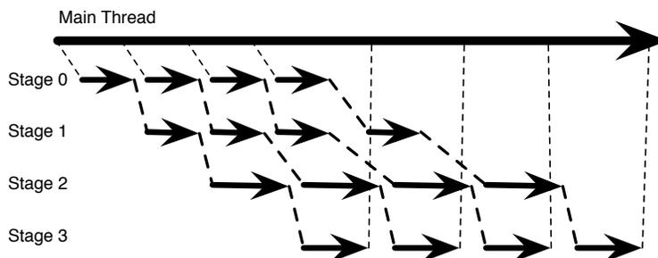
**Figure 4** - Thread Behavior of the Pipeline Programming Pattern
