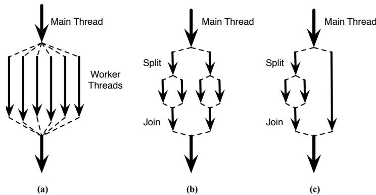
**Figure 2** - Thread Behavior of Task Centric Patterns<sup>1</sup> (a) Task Parallel (b) Symmetric Divide and Conquer (c) Asymmetric Divide and Conquer
