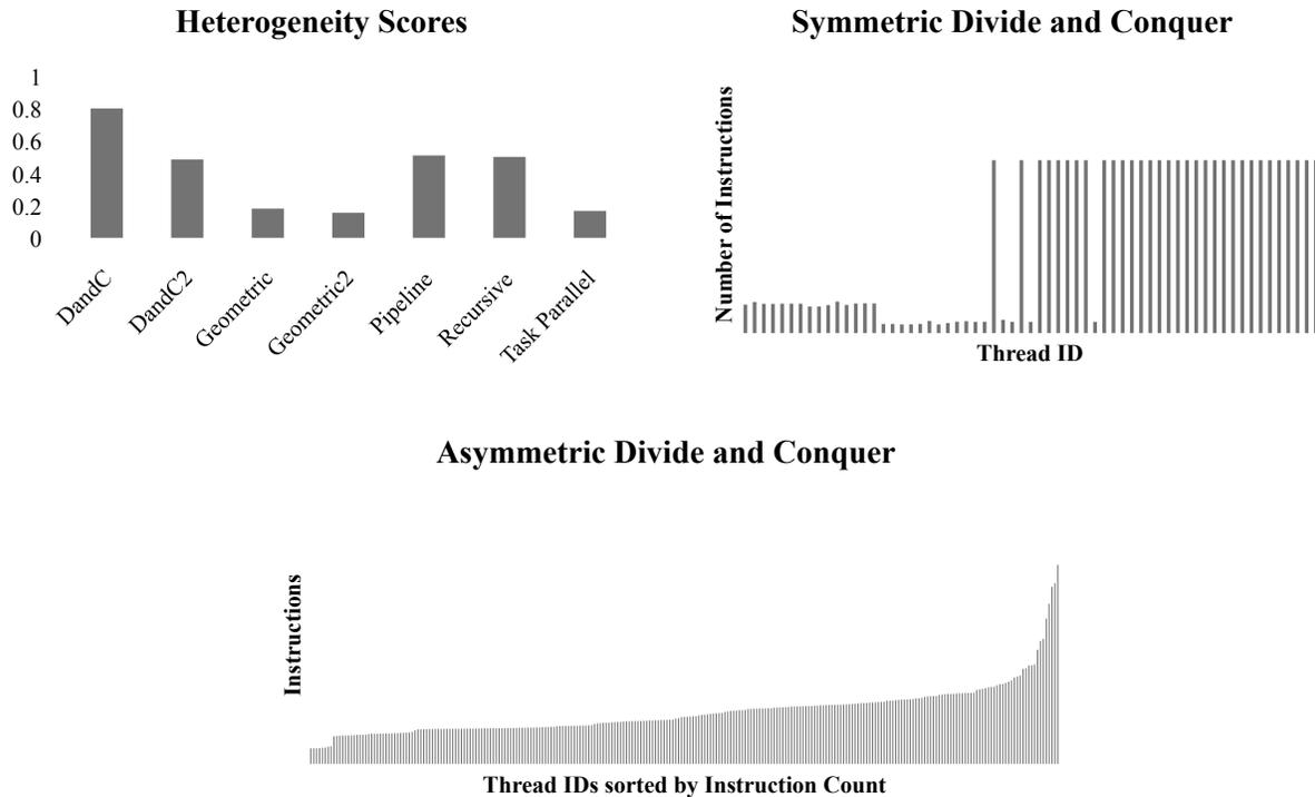
**Figure 5** - Pattern Heterogeneity – top left: Heterogeneity Scores – top right: Symmetric Divide and Conquer thread behavior – bottom: Asymmetric Divide and Conquer thread behavior
